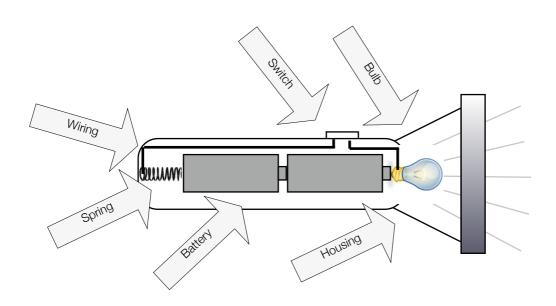
Perform a System FMEA for the flashlight architecture, given the following possible failure modes:
