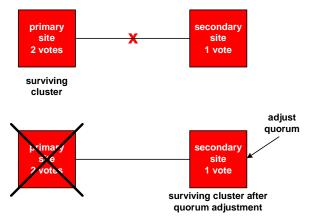
intervention is needed to change the quorum value to that of the votes held by the surviving site. At this point, the secondary system will take over processing. In a lights-out operation, the lightsout site should be the primary site since it may be difficult to get to it to manually adjust quorum.
