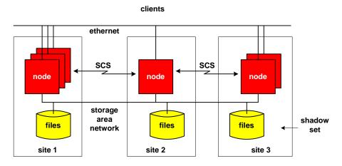
An application can be distributed across several nodes, and users can use any instance of an application on any node. To support shared-everything, OpenVMS clusters provide a Distributed Lock Manager that manages lock requests and a Connection Manager that manages the reconfiguration of the cluster should there be a failure. The Connection Manager ensures that there will not be two cluster subsets actively processing in a split-brain mode.
