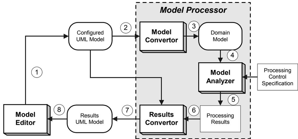
Figure 10-2 A simplified system without a model configurer
