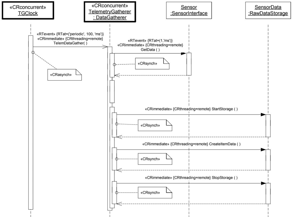
Figure 6-2 Use of Concurrency Model - Synchronous Case
