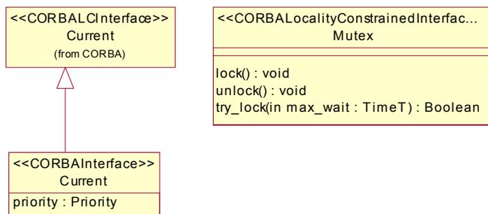
Figure B-10 RTCORBA::Current and RTCORBA::Mutex interfaces
