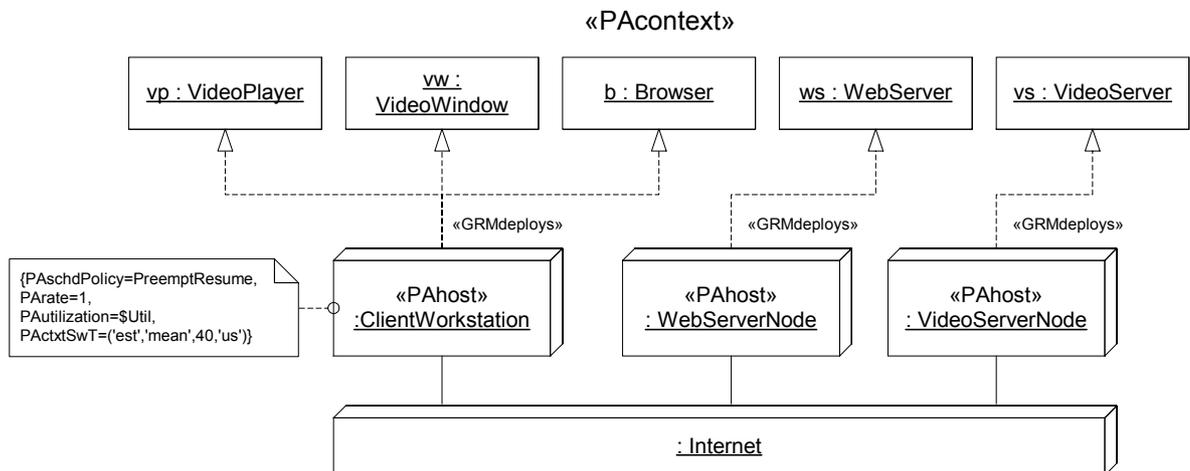
Figure 8-11 Annotated deployment model for the web video application
