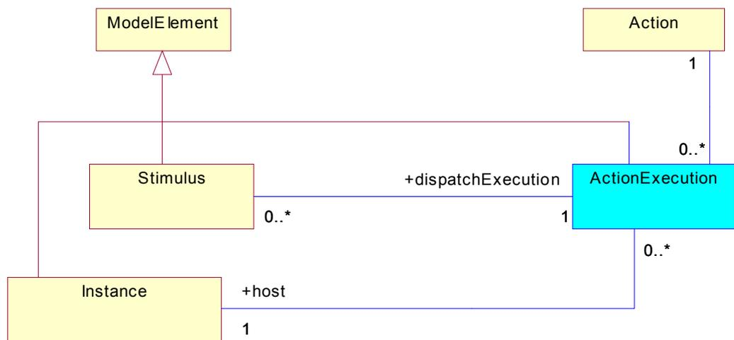
Figure 4-20 Proposed changes to the UML metamodel (ActionExecution)
