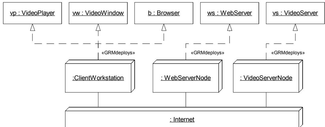
Figure 8-4 The deployment structure of the web video application
