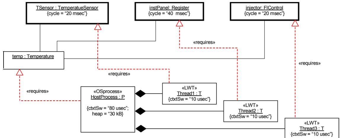
Figure 4-19 Complete system specification for the example
