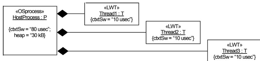
Figure 4-18 Example of a required environment specification
