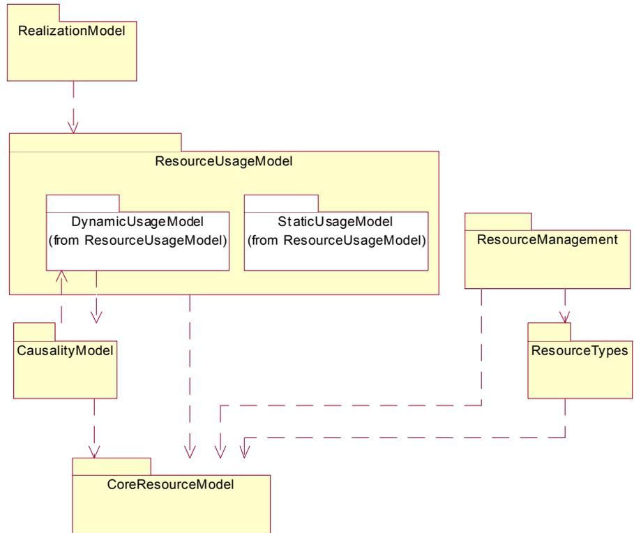
Figure 4-2 Structure of the general resource modeling framework
