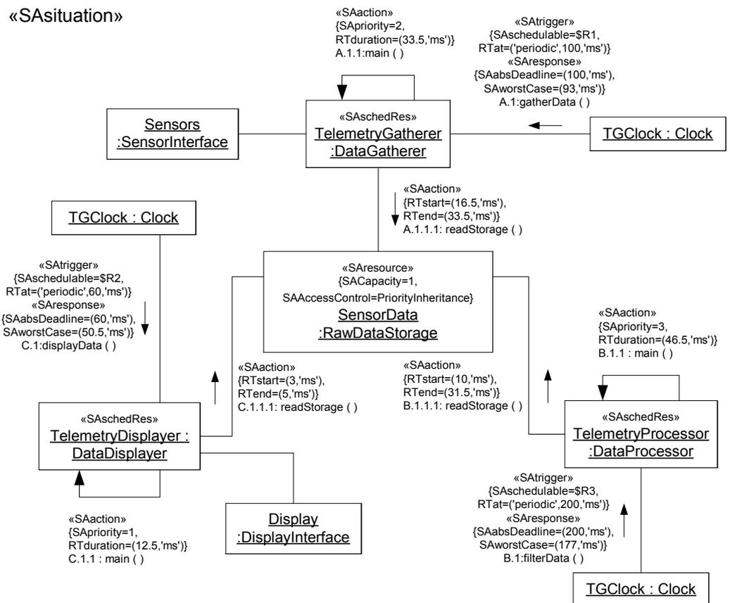
Figure 7-6 A Collaboration Diagram showing all of the schedulable triggers and responses
