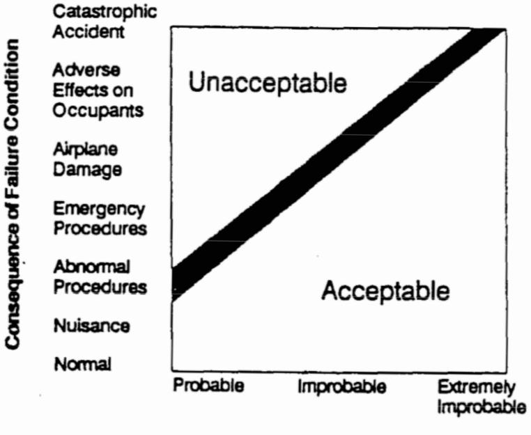
**Probability of Failure Condition**
